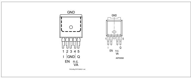
Figure 2 Pin Configuration (top view)
