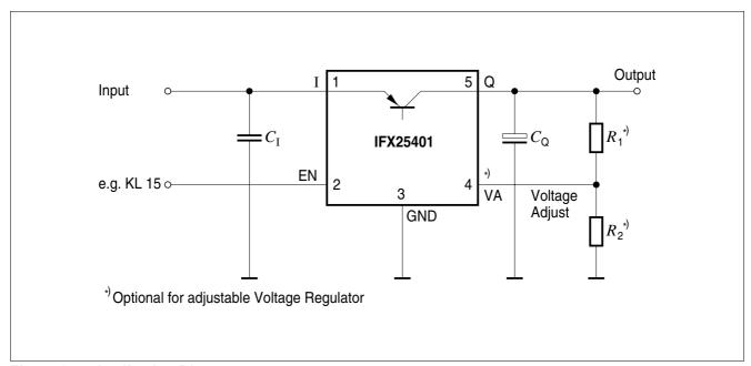
Figure 3 Application Diagram
